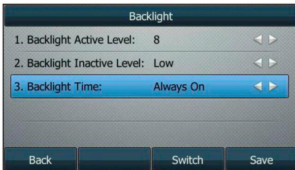
5. Press the **Save** soft key to accept the change or the **Back** soft key to cancel. Backlight is configurable via web user interface at the path **Settings->Preference**.
