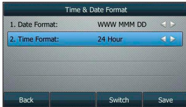
4. Press the **Save** soft key to accept the change or the **Back** soft key to cancel. There are 7 available date formats. For example, for the date format —WWW DD MMM,
